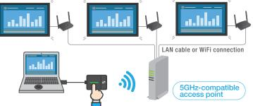
Multicast function for sharing video and audio from a single transmitter to multiple receivers
