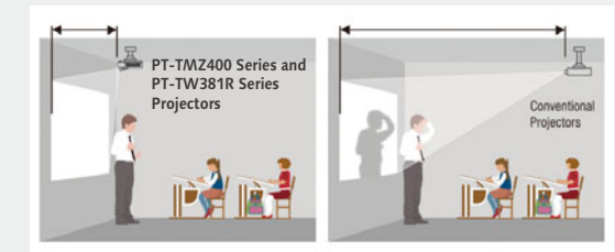
1: Projection distance is 73 cm for the PT-TMZ400/TMW380, 75 cm for the PT-TMX380 and PT-TX440/PT-TX350, and 80 cm for the PT-TW381R/PT-TW380 when projecting an 80-inch image.
